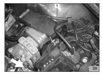
Route Mecanyl fuel line (40/1) downwards as shown in Fig. 40 in the area around the brake lines on the ABS unit
