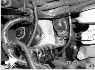
Attach Mecanyl fuel line and metering pump wiring harness (41/1) to the original vehicle brake line using a cable tie
