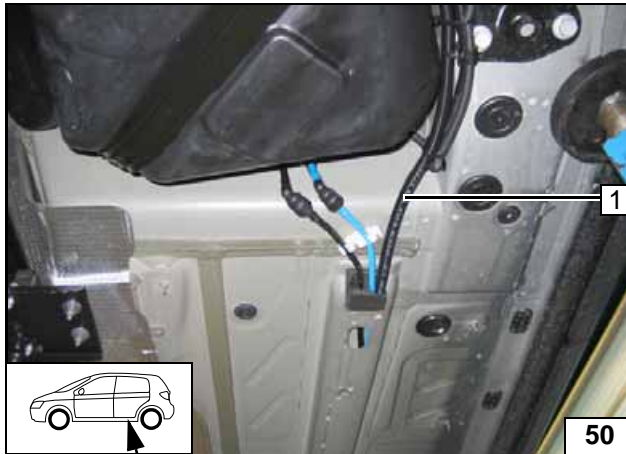
1 Fuel line and wiring harness of metering pump in corrugated tube
