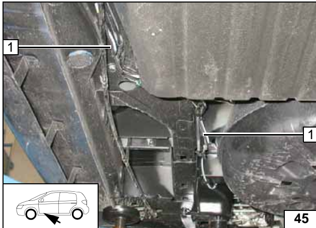
1 Fuel line, metering pump wiring harness
