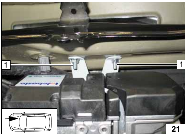
1 M6x20 bolt, flanged nut [2x]
