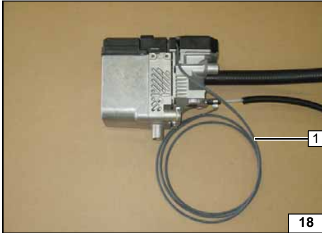
1 Adapter cable of circulating pump
