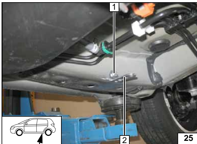
1 M6x20 bolt, spring lockwasher 2 Perforated bracket
