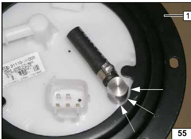
Cut out mounting flange 1 in area of marking
