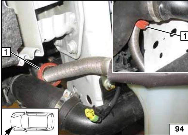
Align spacer bracket 1 with charge-air hose.
