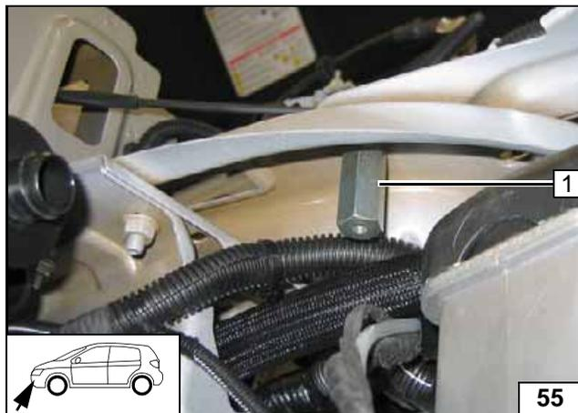
Install M6x40 spacer nut 1 to original vehicle bolt.
