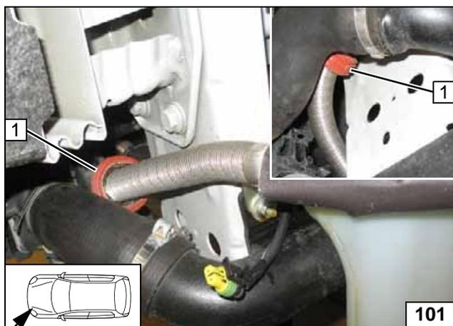
Align spacer bracket **1** with charge-air hose.
