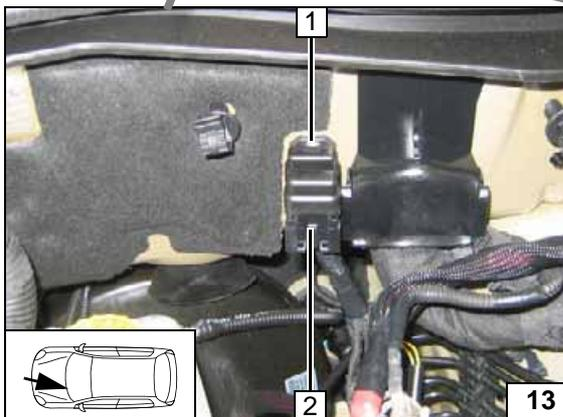
**Engine compartment fuse holder up to model year 2014**
