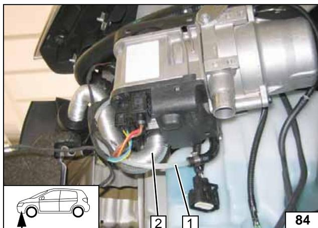
Route fuel line 1 and wiring harness of metering pump to the engine compartment and onto the underbody along original vehicle lines.
