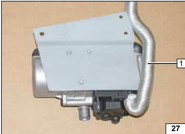
1 Combustion air pipe
