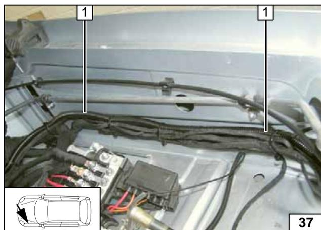
Route fuel line and wiring harness of metering pump in corrugated tube 1 to the firewall and further to the original vehicle lines of the underbody. Attach corrugated tube 1 with wiring harness of heater and earth wire on original vehicle wiring harness with cable ties.
