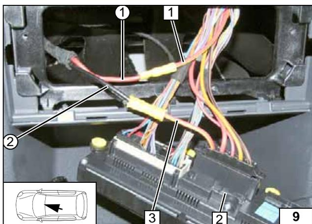
Connection of the 5-pin connector T5e 2 of the A/C control panel. Produce connections as shown in wiring diagram.
