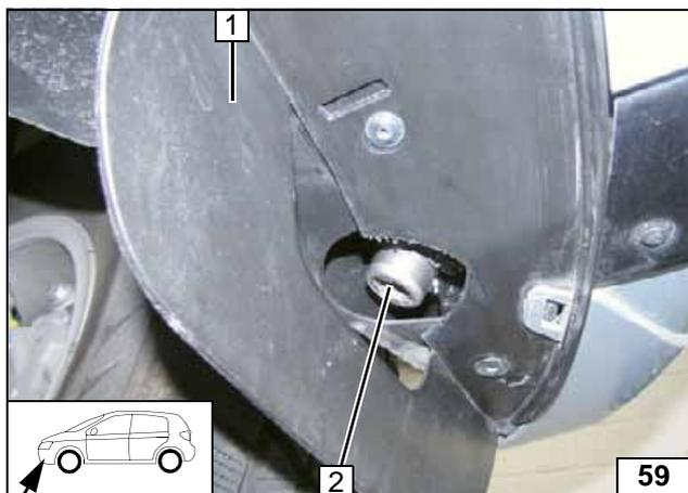
Install bumper 1. Align exhaust end section 2 to the back and flush on the bumper 1. Ensure sufficient distance from neighbouring components, especially from the exhaust system to the bumper, correct if necessary.
