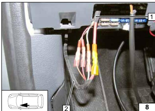
Connect the wiring harness of the fuse holder in passenger compartment 1 to the wiring harness of heater 2 according to the wiring diagram, with same colour wires connected to each other.
