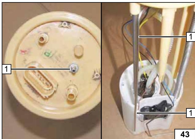
Shape fuel standpipe 1 according to template, cut to length and install.
