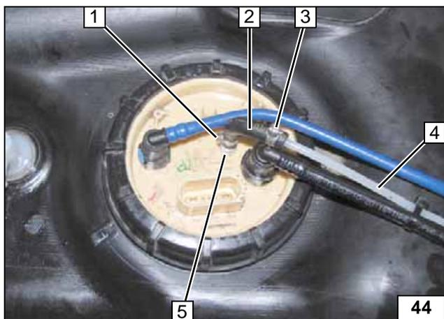
Install fuel-tank sending unit according to manufacturer's specifications.
