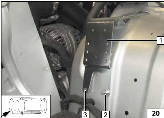
Bend bracket 1 according to the template, loosely install and align vertically.
