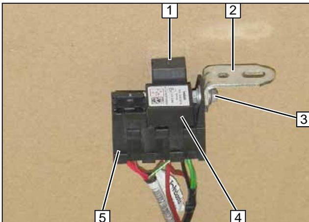
Engage K1 relay socket with fuse holder of passenger compartment 5.
