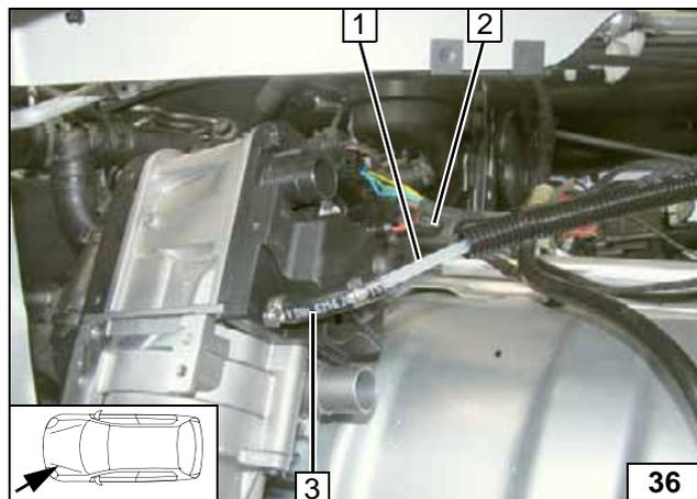
Insert fuel line 1 and wiring harness of metering pump 2 in corrugated tube 2100 and install in the engine compartment.
