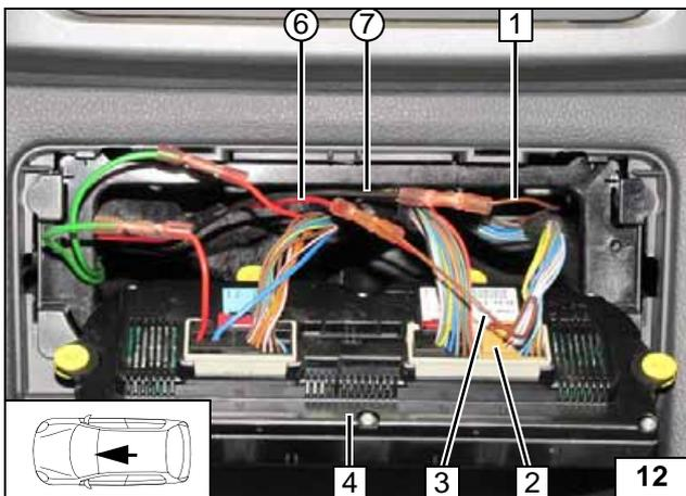
Connection to 16-pin T16m connector **2** Pin 15 from A/C control unit **4**. Produce connections as shown in wiring diagram.
