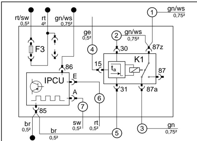
Connect wires to IPCUC socket and K1 relay according to wiring diagram.
