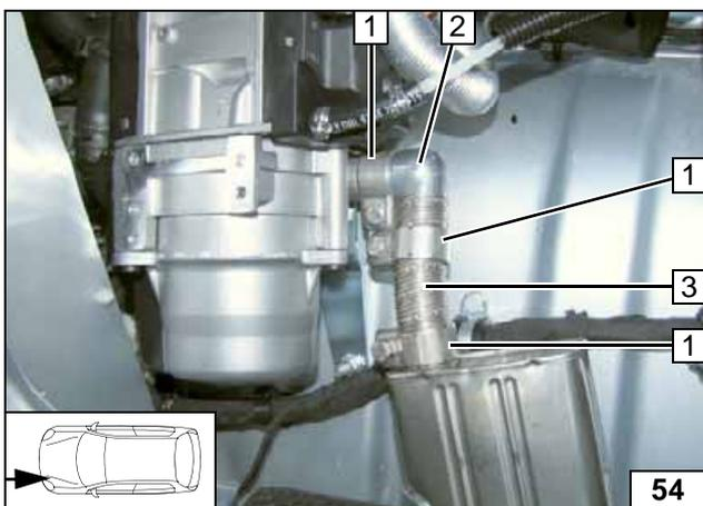
Ensure sufficient distance to wiring harness.
