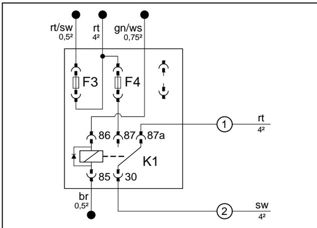
Install F4 25A fuse and K1 relay.
