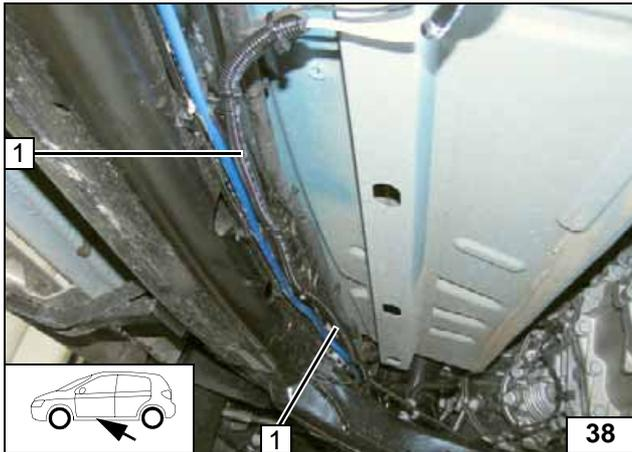
Route fuel line and wiring harness of metering pump in corrugated tube **1** to original vehicle lines at the installation location of the metering pump.
