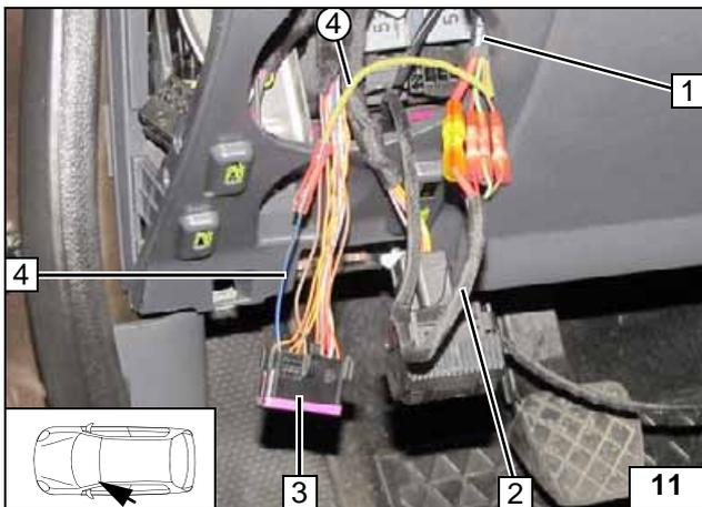
Connect the wiring harness of the fuse holder in passenger compartment **1** to the wiring harness of heater **2** according to the wiring diagram, with same colour wires connected to each other. Connection to OBD connector **3** terminal 15. Produce connections as shown in wiring diagram.
