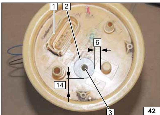
Remove fuel-tank sending unit 1 in accordance with manufacturer's instructions.
