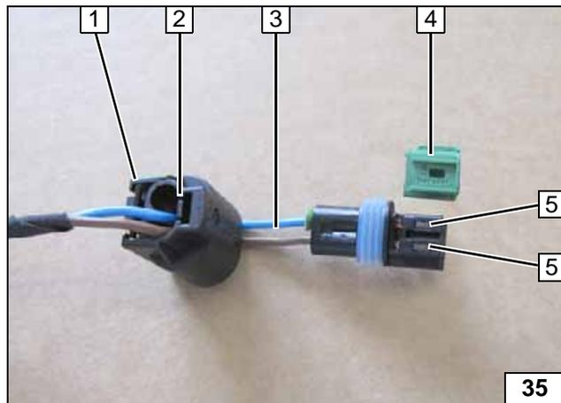
Complete connector of metering pump again after routing. Pin assignment is not relevant.
