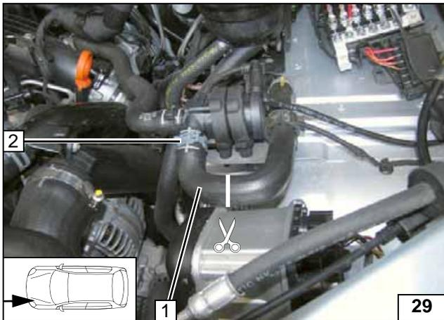
Remove hose section 1 of original vehicle circulating pump / heat exchanger inlet. Hose section 1 and original vehicle spring clip 2 will be re-used.
