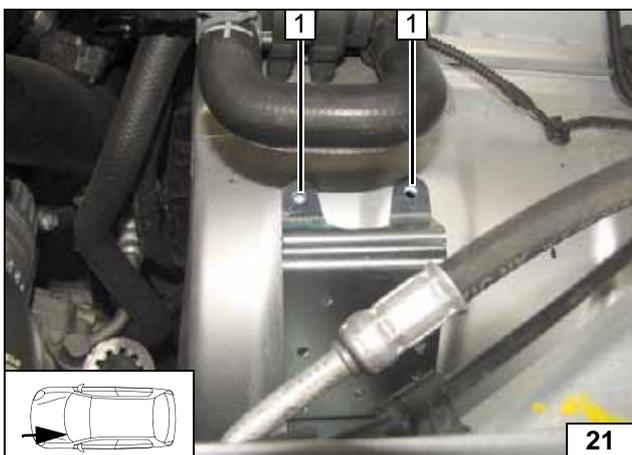
1 Copy hole pattern, 7 mm dia. hole [2x]
