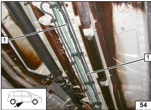
1 Fuel line, metering pump wiring harness in corrugated tube
