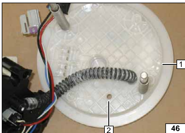
Remove the fuel tank in accordance with the manufacturer's instructions. Remove and dismount fuel-tank sending unit 1 according to manufacturer's instructions.
