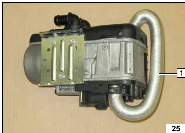
1 Combustion air pipe
