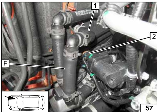
Ensure sufficient distance in 1.8 P (at least 20mm) between original vehicle connector 2 and hoses, correct if necessary.
