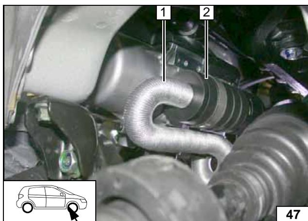
Tighten 5x13 self-tapping bolt on heater (hidden).
