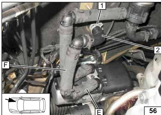
Align hoses. Ensure sufficient distance from neighbouring components, correct if necessary.
