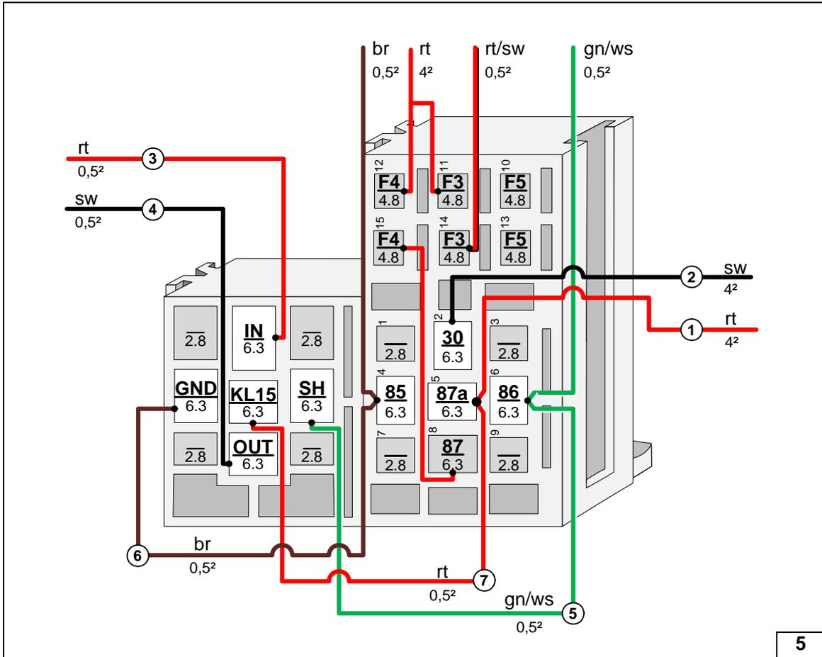
Interlocking PWM GW socket with passenger compartment relay and fuse holder, connecting wires
