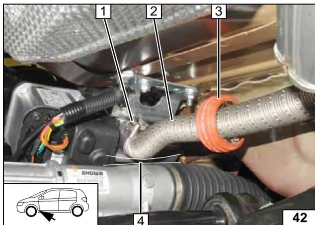
Ensure sufficient distance (at least 20 mm) between exhaust pipe **2** and steering gear at position **4**, correct if necessary.
