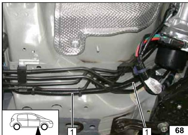
Route fuel line and wiring harness of metering pump in 10mm dia. corrugated tube 1 along original vehicle fuel lines to installation location of metering pump.
