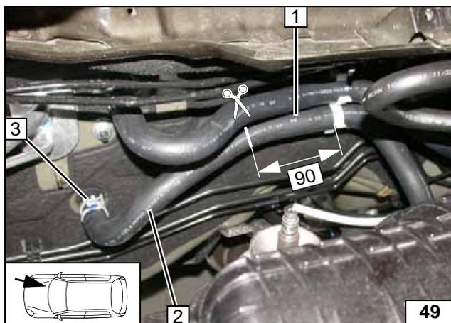
Cut hose of engine outlet / heat exchanger inlet at the marking. Original vehicle spring clip **3** will be reused.
