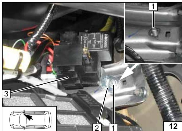
Install premounted angle bracket 2 on original vehicle stud bolt 1.
