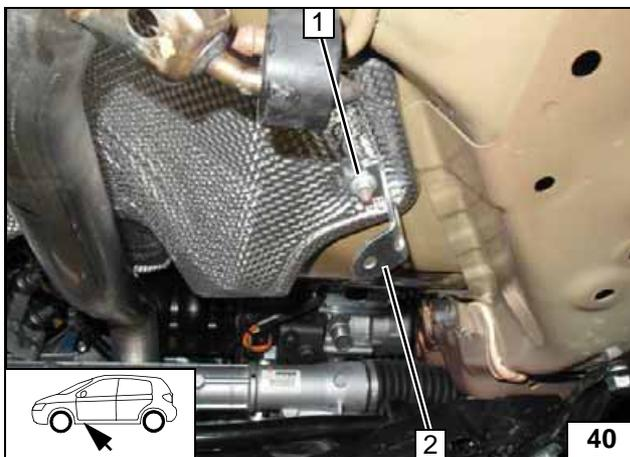
Connect perforated bracket 2 on original vehicle flanged nut in position 1.
