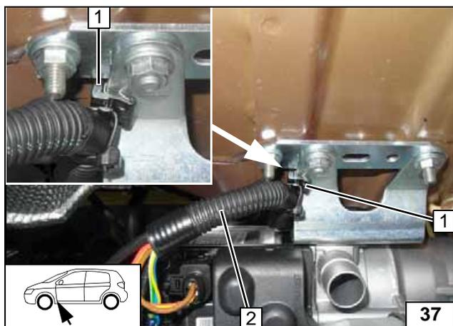
Cut 13mm dia., 250mm long corrugated tube 2 to length and slide over wiring harnesses of heater, circulating pump, metering pump and over fuel line.
