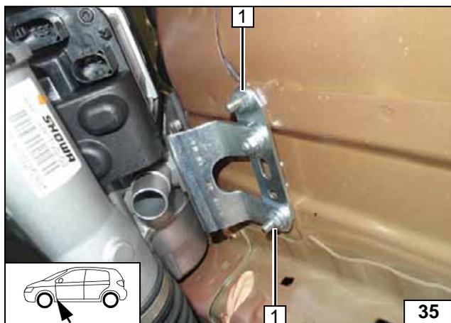
Align heater, tighten bolts of bracket.
