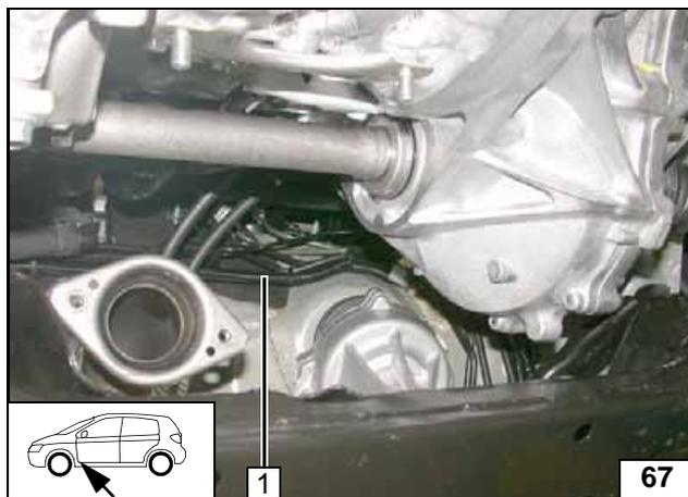
Slide 10mm dia. corrugated tube 1 over fuel line and wiring harness of metering pump and route to the underbody.
