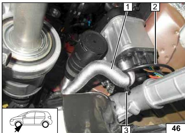
Route fuel line 2 over combustion air pipe 1 and secure using cable tie 3. Ensure sufficient distance from steering gear!
