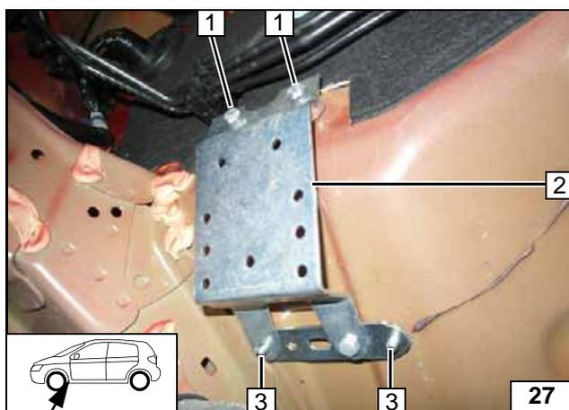
Attach bracket 2 in position 3 [2x] and mount loosely in position 1 [2x]. Align and remove bracket 2 if necessary.
