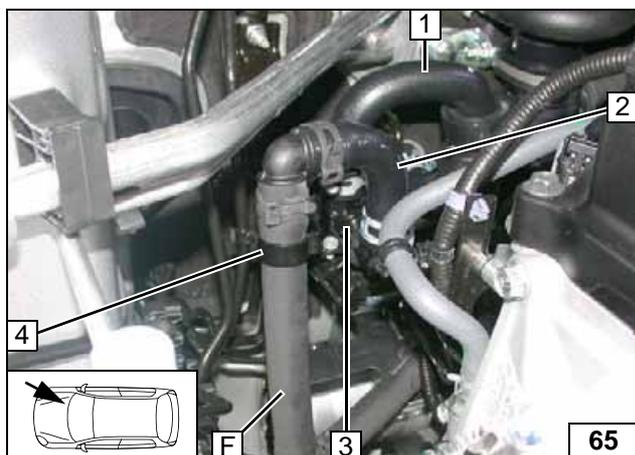
Mount original vehicle circulating pump 3 and hose of heat exchanger inlet 1. Align hoses. Ensure sufficient distance from neighbouring components, correct if necessary.
