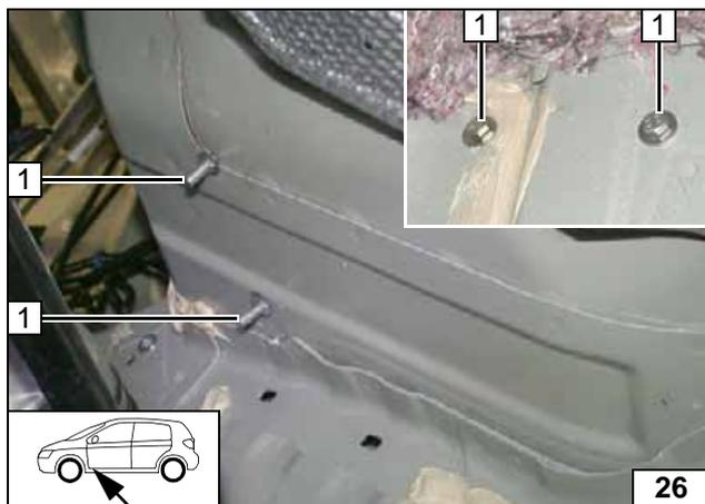
Insert bolts from the passenger compartment.
