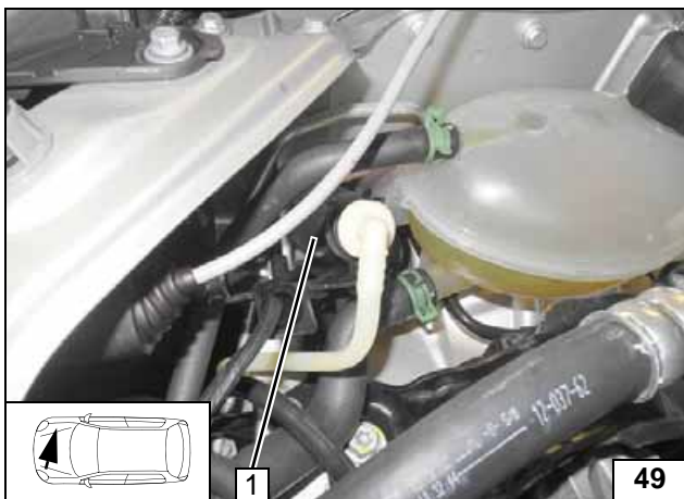
Variant 1: Vehicles with manual supply pump! Fuel extraction with T-piece in fuel supply line! Variant 2: Vehicles with electrical pre-feed pump in fuel tank! Fuel extraction with fuel standpipe in the lid of the fuel supply unit!
