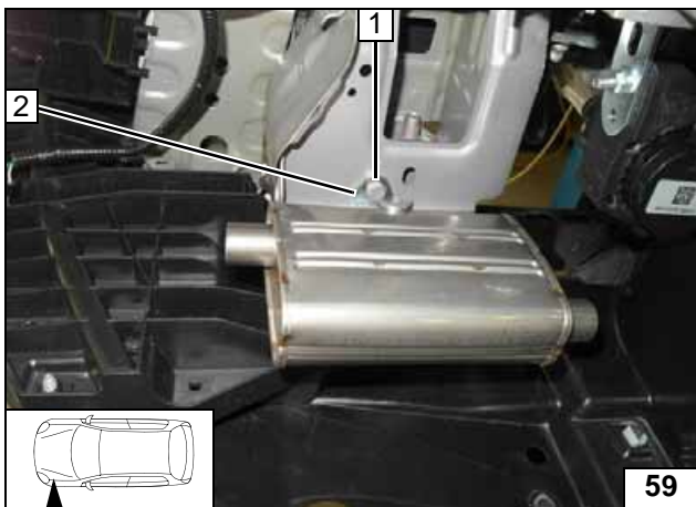
1 M8x20 bolt, spring lockwasher, original vehicle threaded hole 2 Perforated bracket
