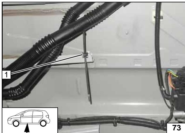
Installing retaining clip
