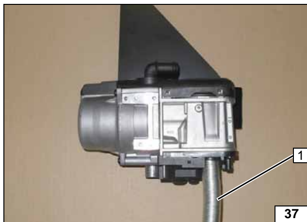
1 Combustion air pipe
