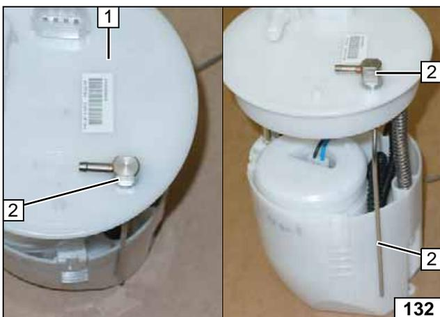
Shape fuel standpipe 2 according to template and cut to length (see follow picture also). Carefully follow separate standpipe installation instruction!
