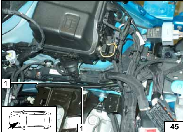
1 Fuel line and wiring harness of metering pump in corrugated tube
