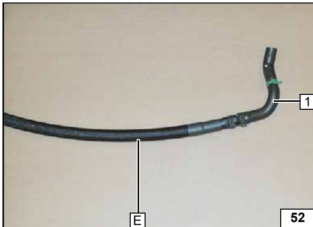
1 Heat exchanger inlet hose section
