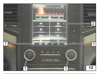
Adjustment of fan speed not necessary, will be automatically set to approx. 1/3!
