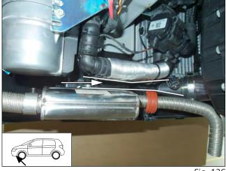
13.2 Mounting exhaust end fastener
