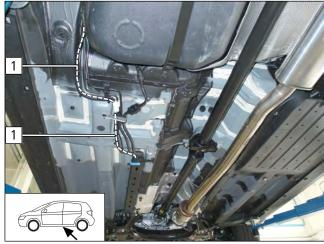
Route fuel line and fuel pump wiring harness in Ø10 corrugated tube 1 along original vehicle fuel lines to fuel pump installation location and secure using cable ties.
