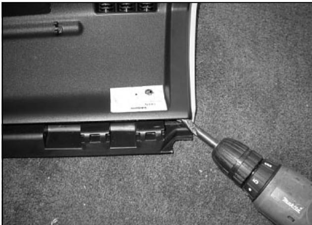
Loch  $\varnothing$  10mm bohren
