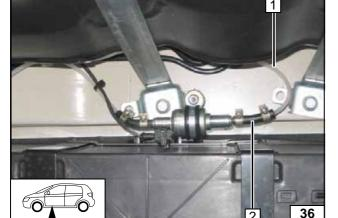
Fuel line from the tank extracting device **1** on the intake side of the metering pump [side without connector].
