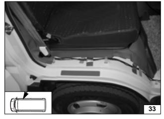
Run combination clock cable harness along original vehicle line
