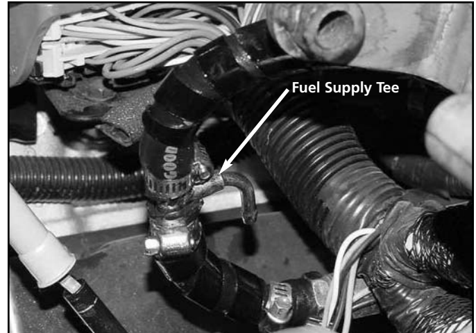
2-27: Fuel Supply Tee Installed
