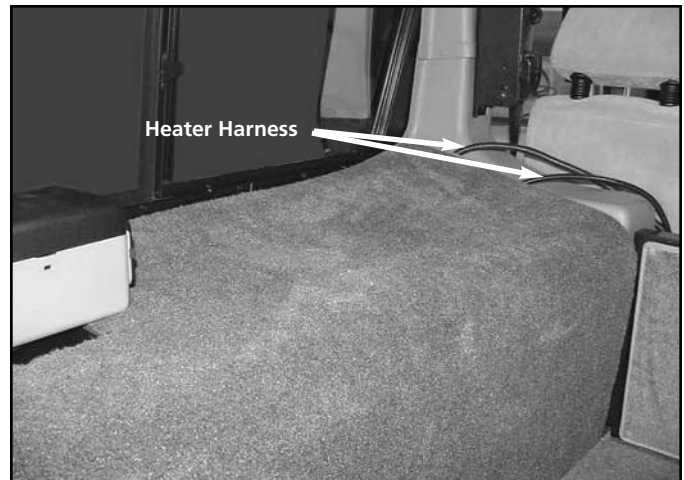
2-9: Carpet In Place - Harness Under Carpet
