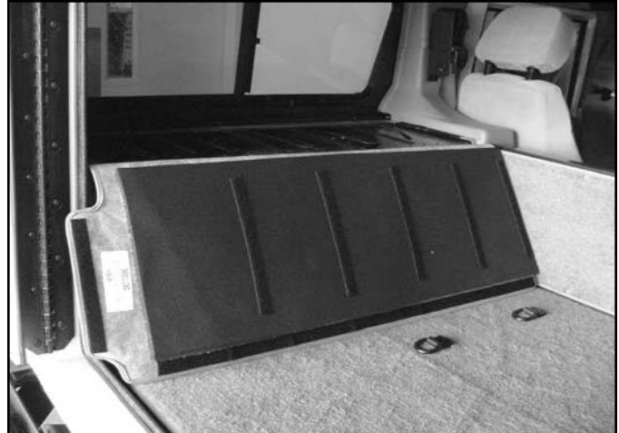
2-3: Floor Carpet Removed
