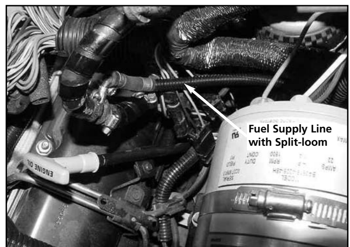
2-29: Heater Fuel Supply Line with Split-loom
