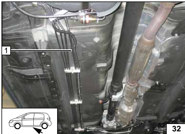
Fuel line and wiring harness of metering pump 1 from center of firewall in 10 mm dia. corrugated tube (2,100 mm).
