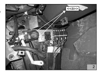
Identify the reserve lines APS C002A and C002D in the vehicle wire harness behind the BSI control unit.
