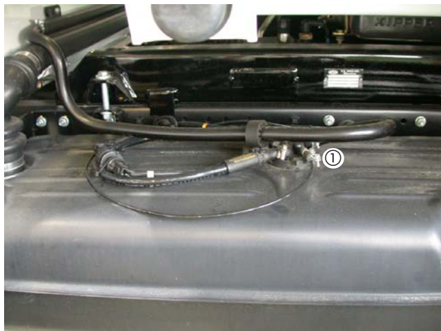
① Steigrohr, eingebaut in der Tankarmatur Rising pipe, installed in the tank fitting
